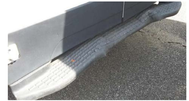
🔄 Rear footboards: Deformations not within economic repair
