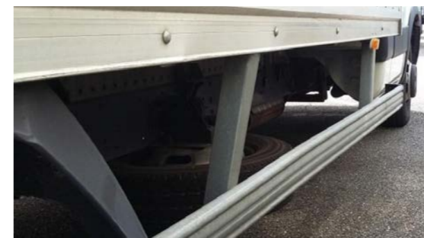
Side underun guards: Deformation within economic repair
