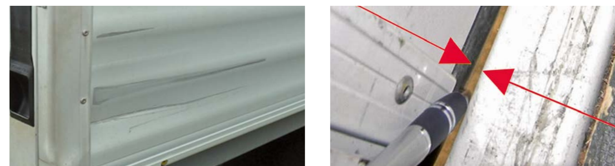
Deformations in the body closures not beyond economic repair, closure not possible or not sand-proof
