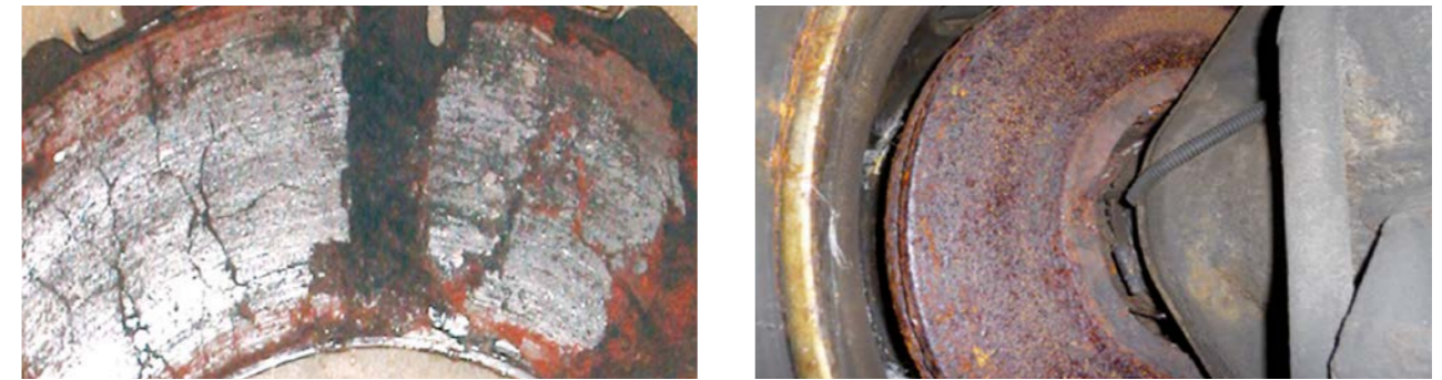
Rusted, ground, worn brake discs
