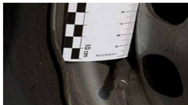
On steel rim: Attachment edge slightly deformed
