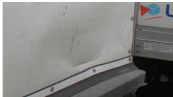
🔧 Side and rear doors: Significant deformation: Repair time > 1 h within economic repair; closure not sealed
