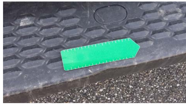
📅 Rear Step Slight deformation
