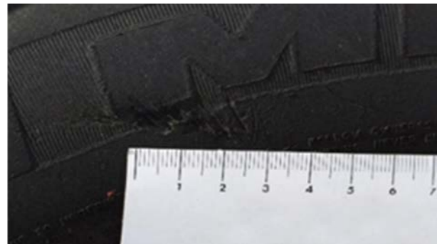
Tyres: Notch \leq 3 mm deep (CONFORMS)
